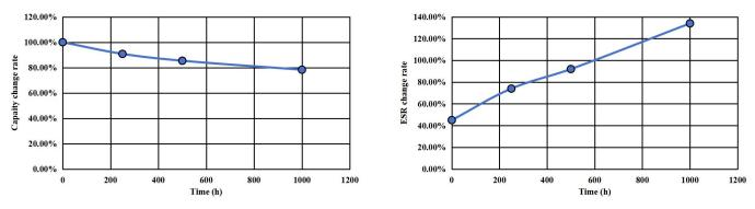
•500-Hour Humidity and Heat Stability (Temperature 40°C, humidity 95%)
